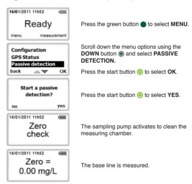
At this point, place the SAF'IR EVOLUTION with the sampling port opening towards the subject to be tested.
