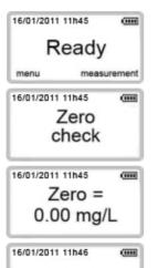
To begin the test, press the start button (1) to select **MEASUREMENT**.
