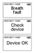
If exhalation is interrupted or if the volume is insufficient, the sampling is aborted. To restart the test, press the start button (a) to select VALIDATE
